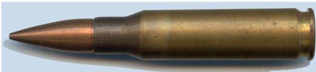
A clean example of annealing marks on the neck of this 7.62mm ball case. It is easily seen where the heat has been applied to the neck thus relieving the stresses built in during manufacture.
