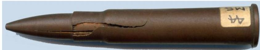
A particularly severe case of season cracking on an Australian .303, even the jacket of the projectile has cracked.
