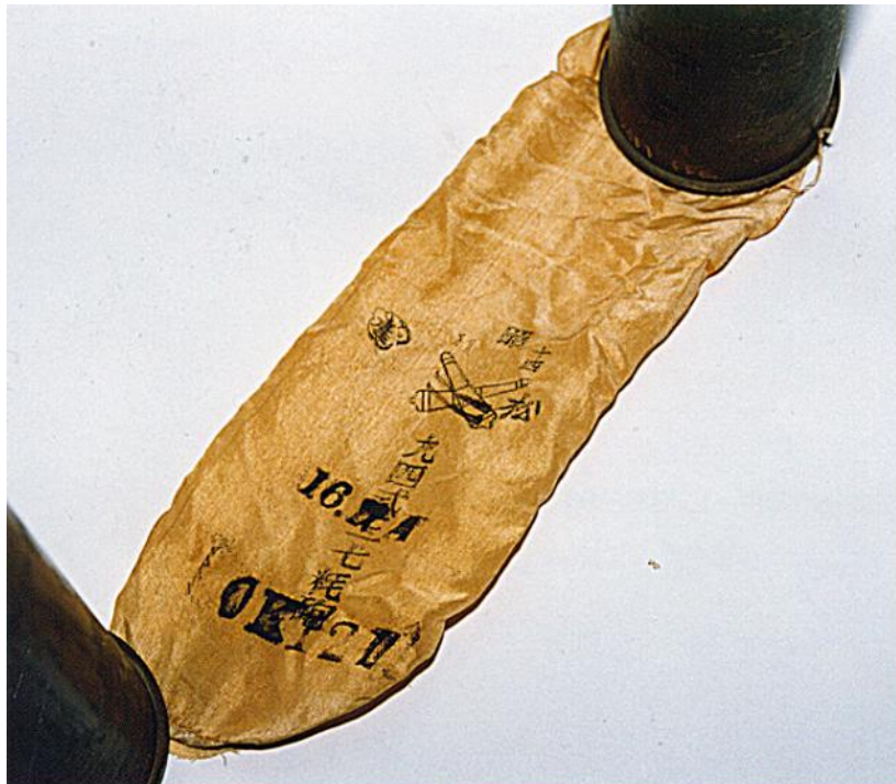
Propellant charge bag for Japanese 37mm showing the propellant details and the crossed cannons of the Osaka arsenal. Photo courtesy of the Australian Logistics training Centre.
