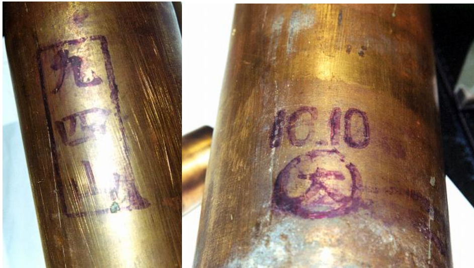
Japanese 47mm cases showing the method of marking the case with propellant information.
