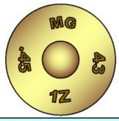
Mk 1Z made at MG in 1943. This model was made from 1943 to 56.
