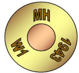
Mk V blank filled at Hendon SA using a reject AP case. Blanks were made here from 1942 to 1945.
