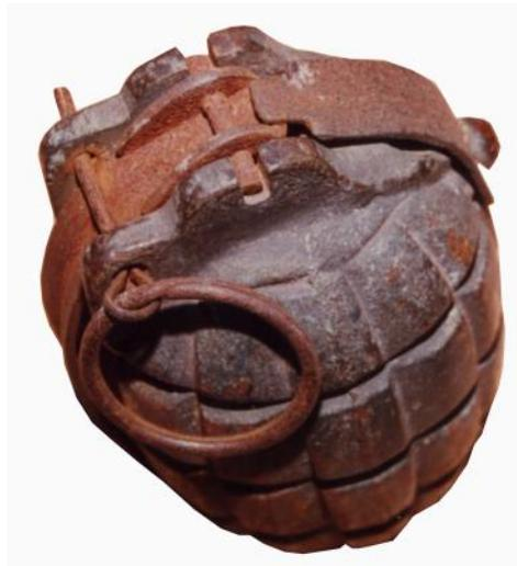
This item was a practice version that was completely empty and was fitted with a spring clip to apply tension to the striker lever. The device was called the "Gibbons patent mechanism". The top version is correctly marked as a drill grenade.
