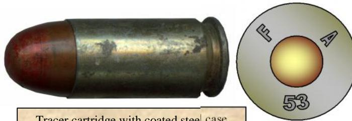
Tracer cartridge with coated steel case and red tip to projectile.
