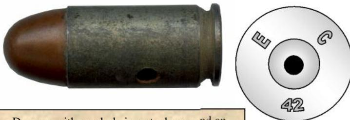
Dummy with one hole in a steel case and an empty primer pocket.
