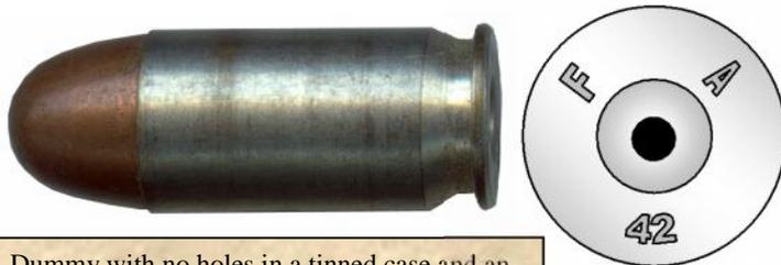
Dummy with no holes in a tinned case and an empty primer pocket.
