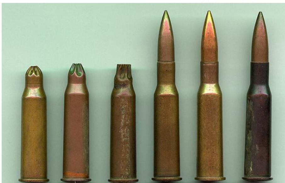
L to R. Finnish blank, Chinese Grenade launcher, Russian blank, American contract ball, Egyptian ball and American contract ball with stained case.
