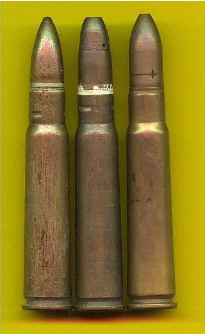
12.7 x 81SR Japanese. Left to right, Tracer, HE/I fuzeless and HE/I fuzeless.
