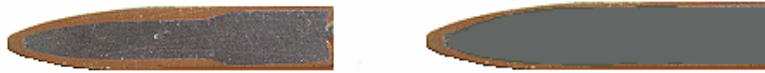
Sectionised 6.5 ball showing left, the strengthened jacket and right the original. The strengthening was to prevent the loss of the core through it.
