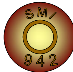
Final model 8x59 with grooved base and embossed headstamp
