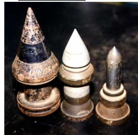
An APCNR shot showing the core on the right and the nose cap in the middle. The complete shot is on the left.
