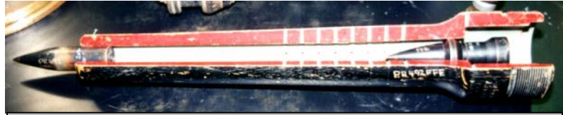
A mock-up of a LittleJohn adapter showing the taper and a shot at either end. The amount of swaging is clearly shown. Photo courtesy of Australian Logistic training Centre.
