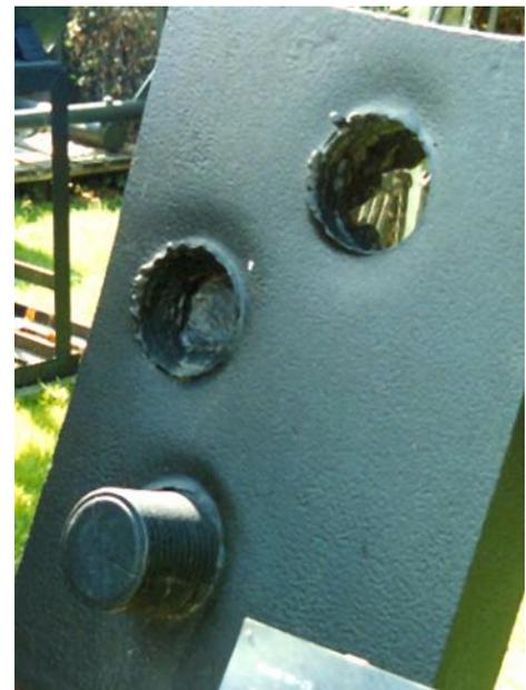
A piece of armour plate showing the effects of AP shot. The top shows a successful penetration, the middle shows a partial and the bottom shows failure with a jam. The two top holes also exhibit the petalling associated with the initial gouging of the plate. Photo courtesy of The Artillery museum Woolwich.
