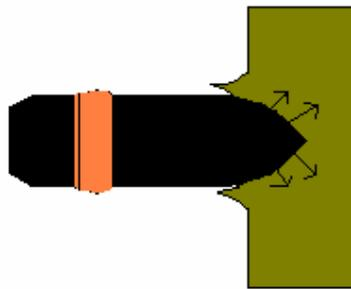
2. As the penetration increases the plastic flow of the metal becomes more difficult; it will cease when the projectile penetrates to about the shoulder region. To penetrate further the projectile needs to cause the plate to flow radially or axially away from the shot. If the armour plate is sufficiently thick and tough at this time the shot will fail to penetrate. The shot will be very tightly jammed in the armour.
