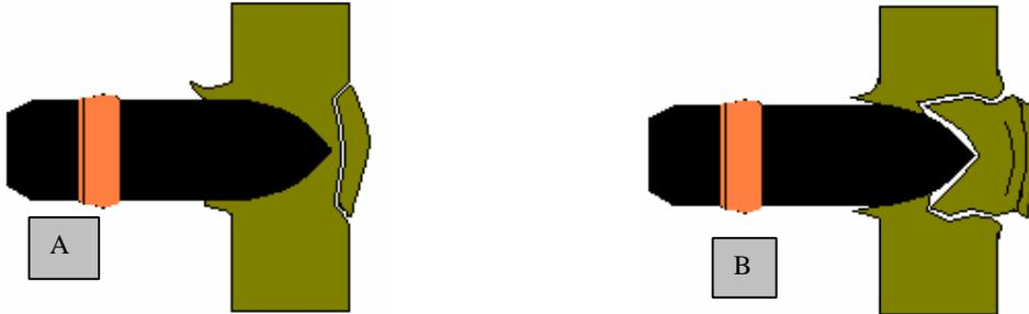
5. Some spalling from the inner face will occur if the shot penetrates to a great depth without actually defeating the armour. This spalling is caused by weaknesses built into the armour plate during manufacture and allows the pieces of armour to fly off into the vehicle.
