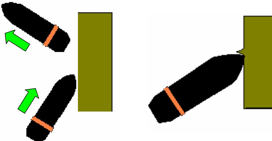
3. The increased resistance provided by the gouging and petalling occurring begins to slow the point of the projectile but the base wants to keep moving thus producing a turning moment around the middle of the projectile. This levering action causes the plate to commence breaking up thus reducing the resistance to penetration. The reduction in resistance also causes the projectile to change its direction in doing so it usually punches out a plug.
