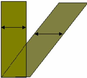
A difficulty for the shot at an angled impact is a simple geometry problem. As the angle changes, the amount of material to penetrate increases. Sloped armour is one of the standard methods of increasing the armour protection of a tank.
