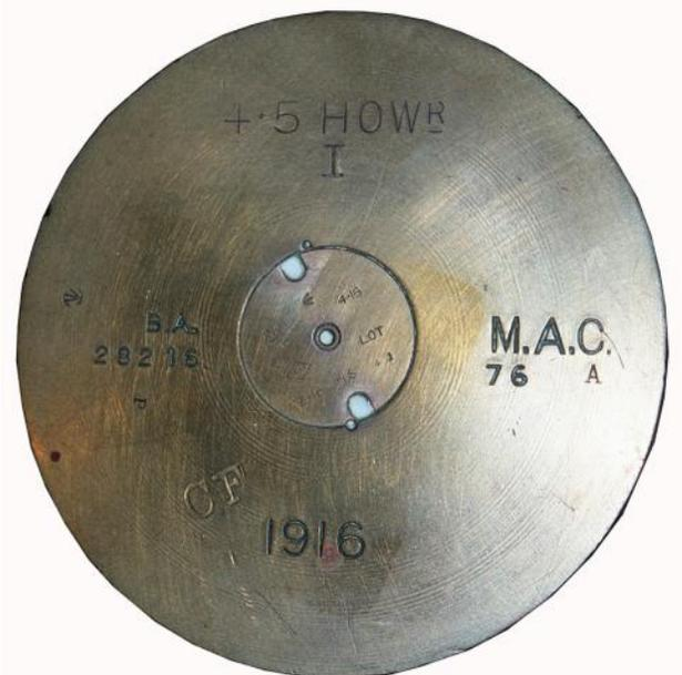
The base of a 4.5inch Howitzer cartridge in very good condition considering its age. The primer was the number 1.
