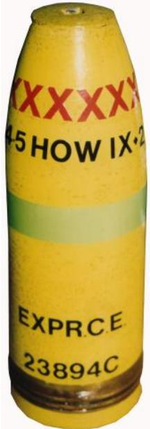
4.5in How filled TNT and marked with a filling ring indicating suitability for universal use.
