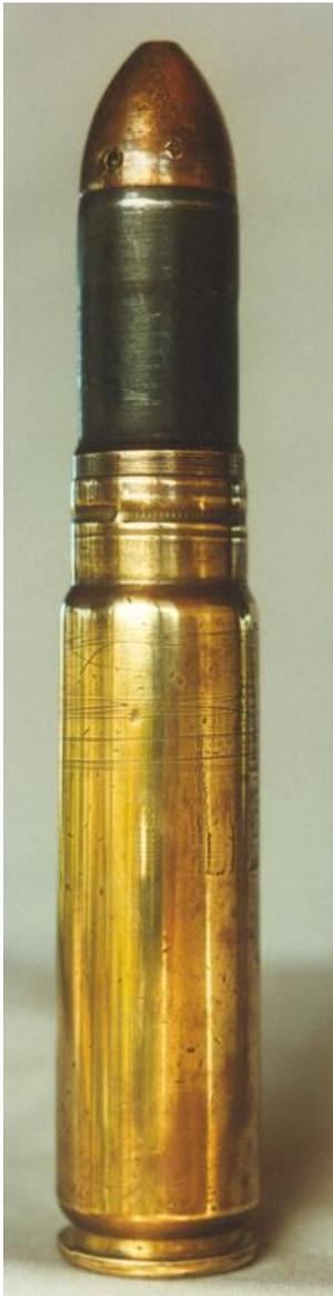
This cartridge was used in weapons developed by Japan as their war experiences taught them what was needed in a weapon and cartridge combination. The case was made from brass and was filled with 21.4 gms of short cord, single-base propellant. It weighed 113.5 gms.
