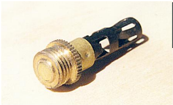
An example of the capped switch that could be used with the time pencil.
