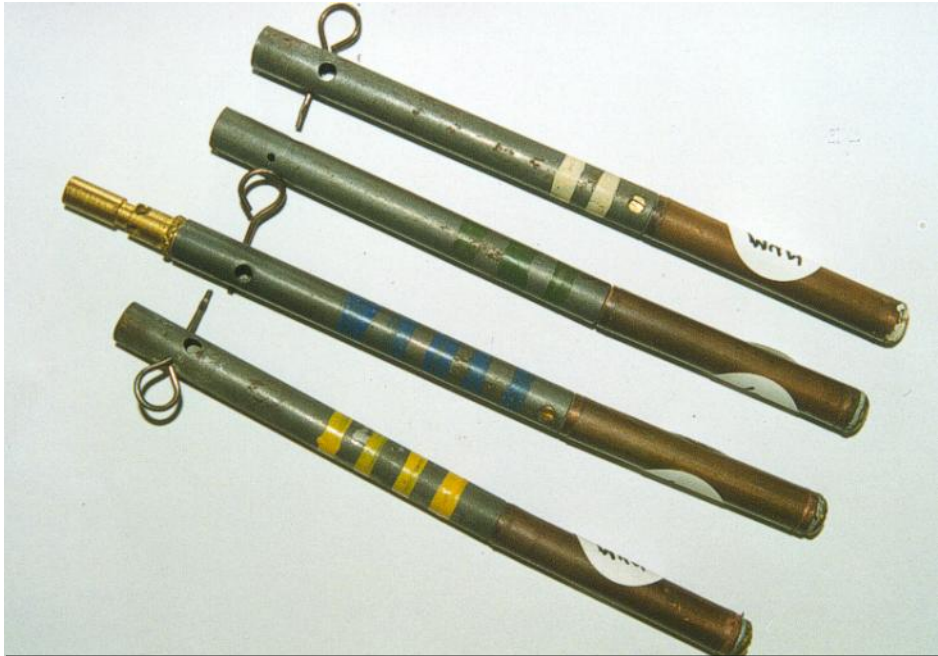
No 10 time pencils showing clearly the delay indication markings.
