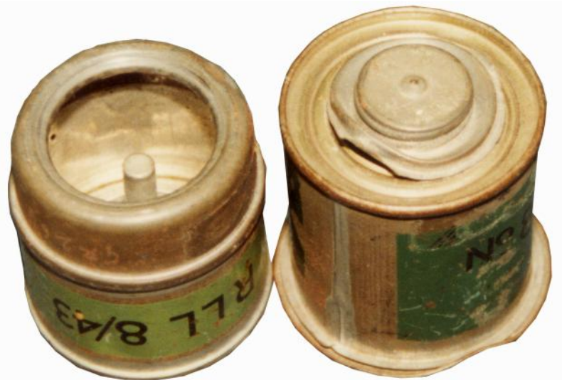
A number 81 grenade separated into the two pieces that make up the grenade. On the left is the top WP portion and on the right is the Hexachlorethane/Zinc portion.
