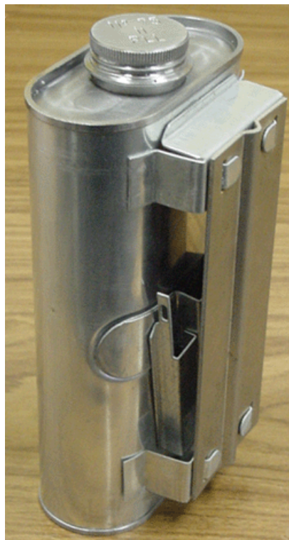
Shown here is the way in which the detonator holders were angled to put the two detonators closer together. This is a replica
