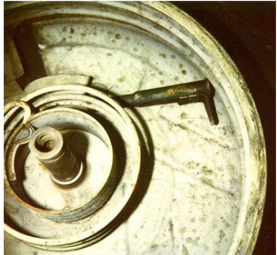
The interior of the Vickers aircraft "K" gun magazine showing the feed device in the pathway in which it slides.
