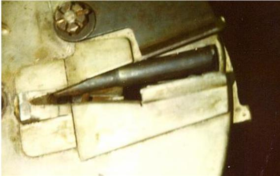
The magazine slot showing the feed device when the magazine is completely empty. Note the chamfer lining up exactly with the slot edge.
