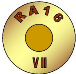
Mk. 7 Ball. Cu/Ni projectile.
