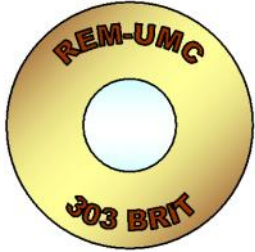
Mk. 7 Ball. Cu/Ni projectile and tinned primer.
