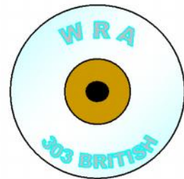
Drill cartridge nickled case empty primer pocket.
