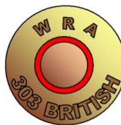
Variations in the headstamp and primer material. The primer annulus colour is wrong as these are ball rounds.
