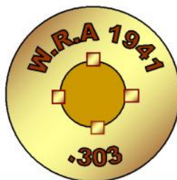
Winchester Repeating Arms Ball Mk. 7 with four very heavy stabs around the primer and a powder blue annulus and one without the colour?
