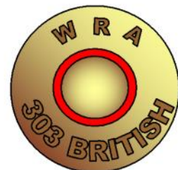
Variations in the headstamp and primer material. The primer annulus colour is wrong as these are ball rounds.
