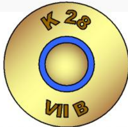
An early incendiary loading as indicated by the "B" after the model number.
