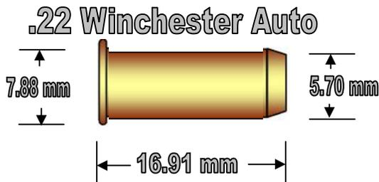
This cartridge was used only in the Winchester model 1903 semi-automatic rifle. The dimensional differences were intended to prevent the use of gunpowder filled cartridges in the semi-auto mechanism.
