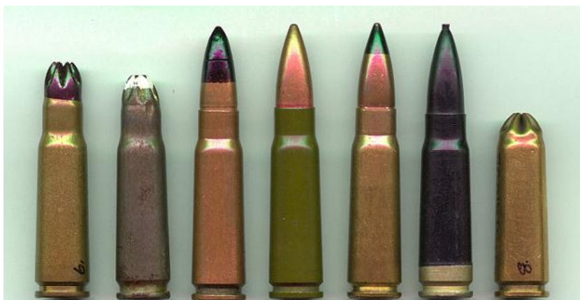
L to R. Egyptian grenade launcher, Polish grenade launcher with Czechoslovak H/S?, Chinese API showing the variation in tip colouring, Chinese ball, Yugoslav ball with black tip?, East German drill and Yugoslav grenade launcher.
