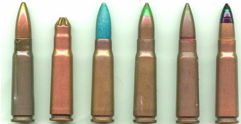
L to R. Czechoslovak drill with steel lacquered case, Unknown grenade launcher with steel case, Finnish wooden bullet with brass case, Russian ball with copper washed steel case and Chinese API with steel case and later colour code of a simple black tip.
