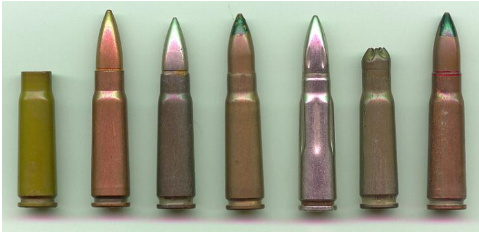
L to R. Chinese showing common olive lacquer, Unknown steel case w/copper wash (probably Chinese), Czechoslovak steel case showing grey lacquer, Egyptian Tracer with brass case, Russian drill cartridge with nicked and fluted case ( Consult the German section to see the influence of German thinking in drill carts) Czechoslovak grenade launcher with steel case and Russian Tracer with steel copper washed case.
