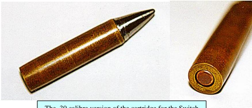
The .30 calibre version of the cartridge for the Switch No. 8 clearly showing an off-centre primer and the absence of any headstamp or primer markings as found on the .40 calibre version. Possibly a fake.
