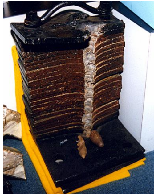
A series of plates perforated by a 6-Inch Beehive with some examples of the slug associated with this type of demolition store. Photo courtesy of the ALTC.
