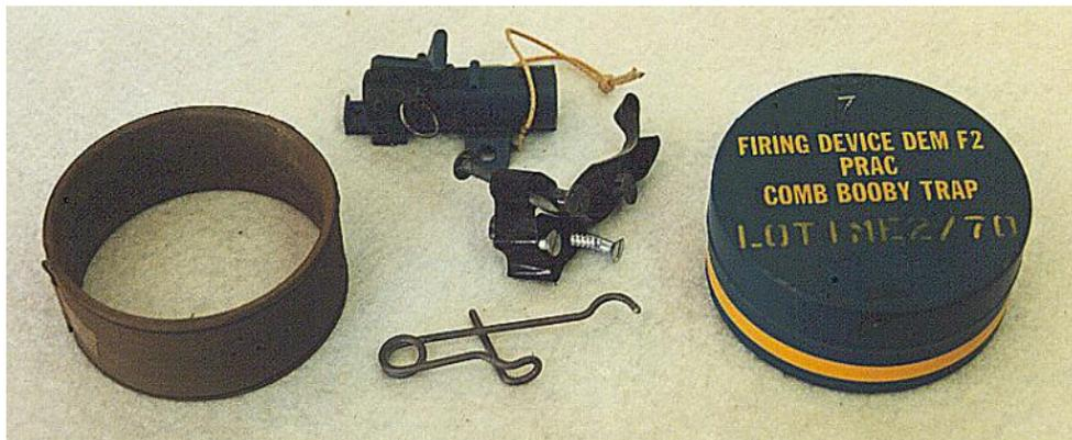
The practice version of the F1A1 firing device. This particular example is incorrectly marked with the yellow band indicating an HE filling. In the foreground is the tension release device.
