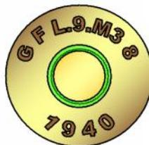
The cartridge is still in production in Italy and elsewhere in the world. It is after all a standard 9mm parabellum and almost everyone makes it. This M38 can be clearly identified by the headstamp shown below. The model number M38 was dropped in 1957.
