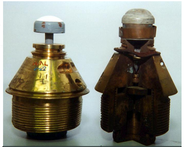
Fuze percussion No. 106 courtesy of ALTC. This one is an Australian version.
