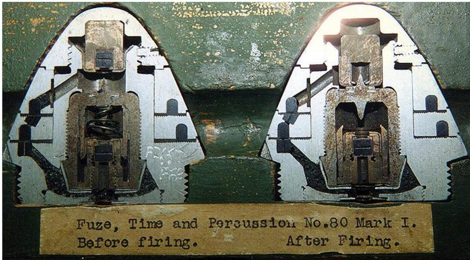
Clearly seen on the right is the movement of the time pellet plug downward onto the needle with the consequent straightening of the stirrup spring lugs, also the downward movement of the ferrule which straightens out the lugs on the percussion element stirrup spring. Photo courtesy of ALTC.
